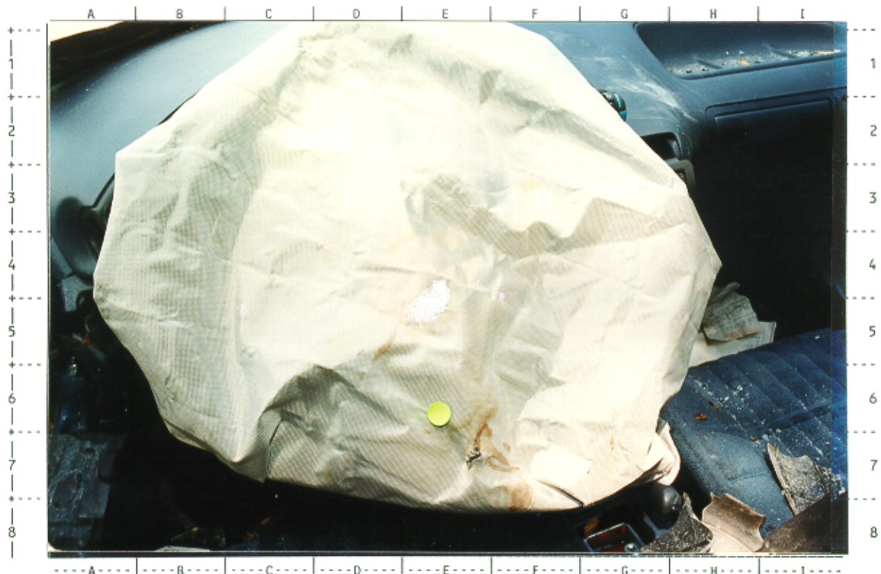
# 54 -- Close-up view of 1991 Chevrolet Corsica's driver air bag with blood smudge and 2.5 centimeter tear
